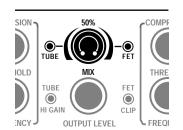
While playing a note on an open string, sweep the MIX Control from the center (Equal Blend of Tube and FET), to the left (100% Tube) and to the right (100% FET.) Between these three positions lie a myriad of unique and outrageous sounds that you will find yourself exploring for many years. The ability to combine two completely separate front end technologies allows you to "custom-build" the pre-amp of your *dreams*, by simply using the MIX Pan Pot.
